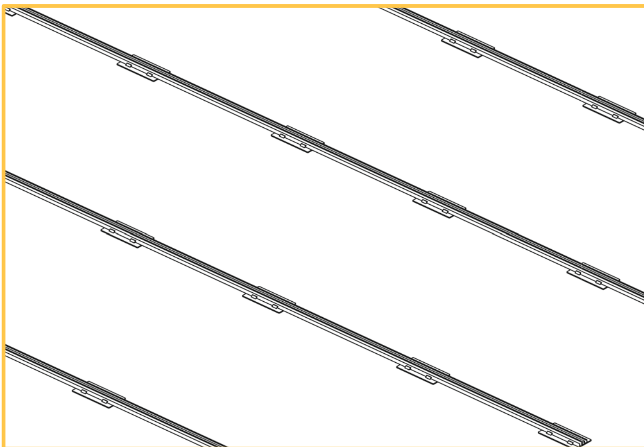
2. u zavisnosti od smera montaže rasporediti aluminijumske šine i zaštitne podloge / depending on the direction of installation, arrange aluminum rails and protective bases
